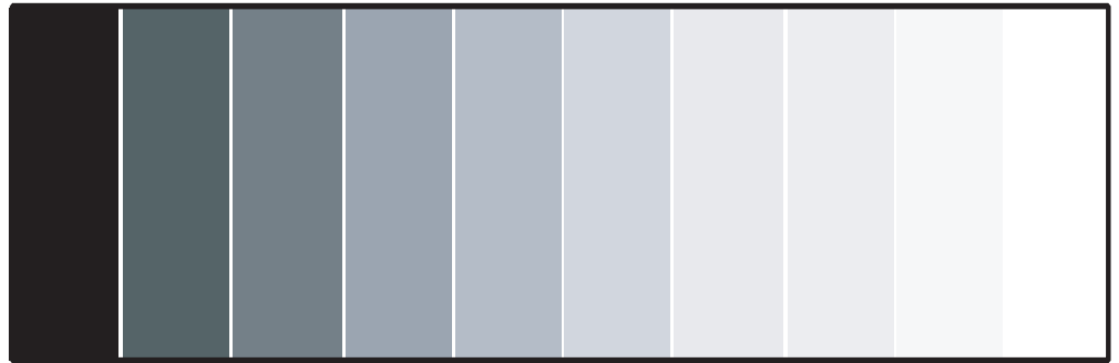
Figure 4-3. Typical Gray Bar Pattern for Adjusting Contrast
